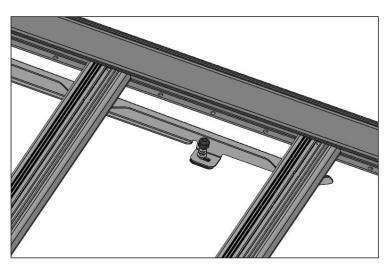
**STEP-6** Fix the bracket with bolt to the holes on the vehicle. Repeat this process for all brackets.
