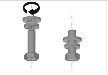
**STEP-4** Attach spring washer first then flat washer to M8x25 hex bolts
