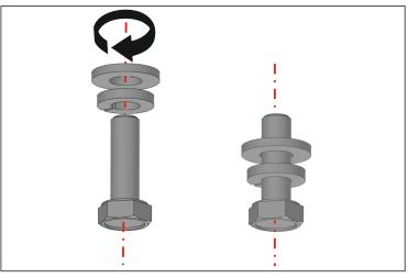
**STEP-4** Attach spring washer first then flat washer to M6x25 hex bolts
