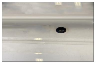
**STEP-1** Remove factory rubber plugs as shown.
