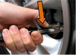
NOTE: ARB's tyre filler attachment is equipped with a stop valve. Air will not pass through the tyre filler attachment until it is connected to a tyre valve.
